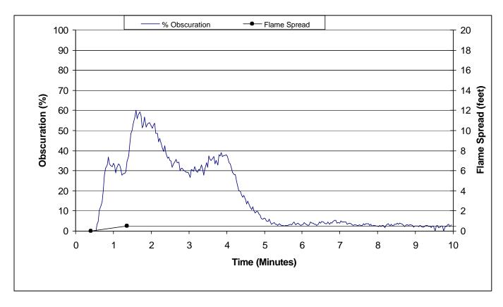
Test No. 2 06CA55853 / SV16584 11140612 Flame Spread Index: 0 Smoke Developed Index: 190 Max. Flame Spread: 0.5
