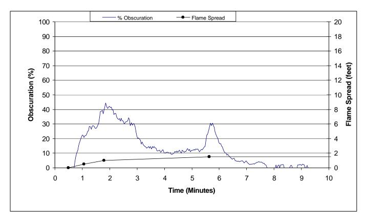
Test No. 1 06CA55853 / SV16584 11140610 Flame Spread Index: 5 Smoke Developed Index: 145 Max. Flame Spread: 1.5
