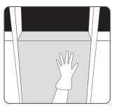
3. Release & expand Once in place, UltraBatt™ insulation naturally expands to fill in the space, creating a snug, custom fit.
