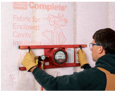
Inspect-R® Density Gauge accurately reads R-values in seconds.
