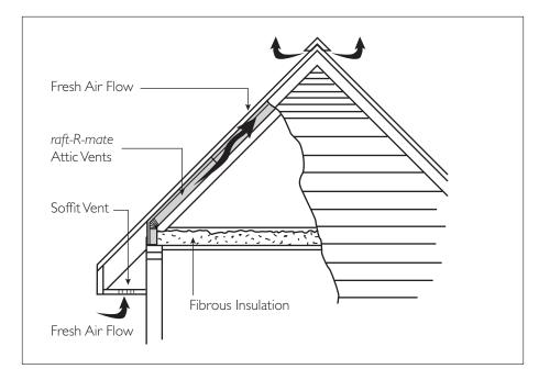
Note: When prolonged outdoor cold temperatures, or higher interior humidity conditions are expected, a vapor retarder, such as asphalt kraft paper, should be installed on the room side of the rafter batt to reduce the intrusion of moisture into the attic or rafter cavity.
