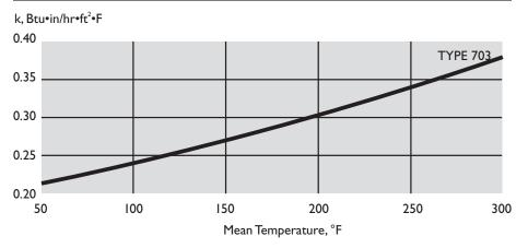
Apparent thermal conductivity curve determined in accordance with ASTM Practice C 1045 with data obtained by ASTM Test Method C 177. Values are nominal, subject to normal testing and manufacturing tolerances.
