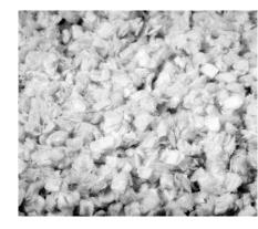
Advanced ThermaCube Plus® loosefill fiber glass insulation offers enhanced engineering and unique cube-shaped bits offering more uniform coverage than standard loosefill. The cube shapes "tumble" into nooks and crevices to provide complete coverage and a smooth finish.
