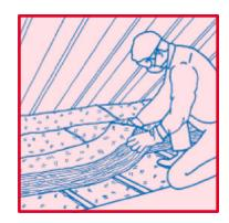
ii. For Lofts with Trusses: Use correct width of insulation for joist spacing. Start insulation at outer edges and work towards centre. Place over top of existing insulation, between and parallel to joists. Cut as needed with a utility knife. Butt ends together carefully to ensure complete coverage.
