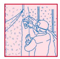
c. A separate vapour control layer should be installed directly over the insulation on the inside facing surface. Overlap its joints by 150 mm and staple every 200 to 300 mm on the face of the wood studs.
