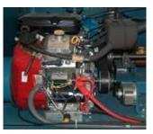
18 hp Briggs & Stratton V-Twin Gas Engine W/Positive Pressure Lubrication System
