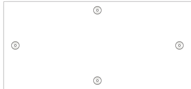
4 Fasteners Per Board
