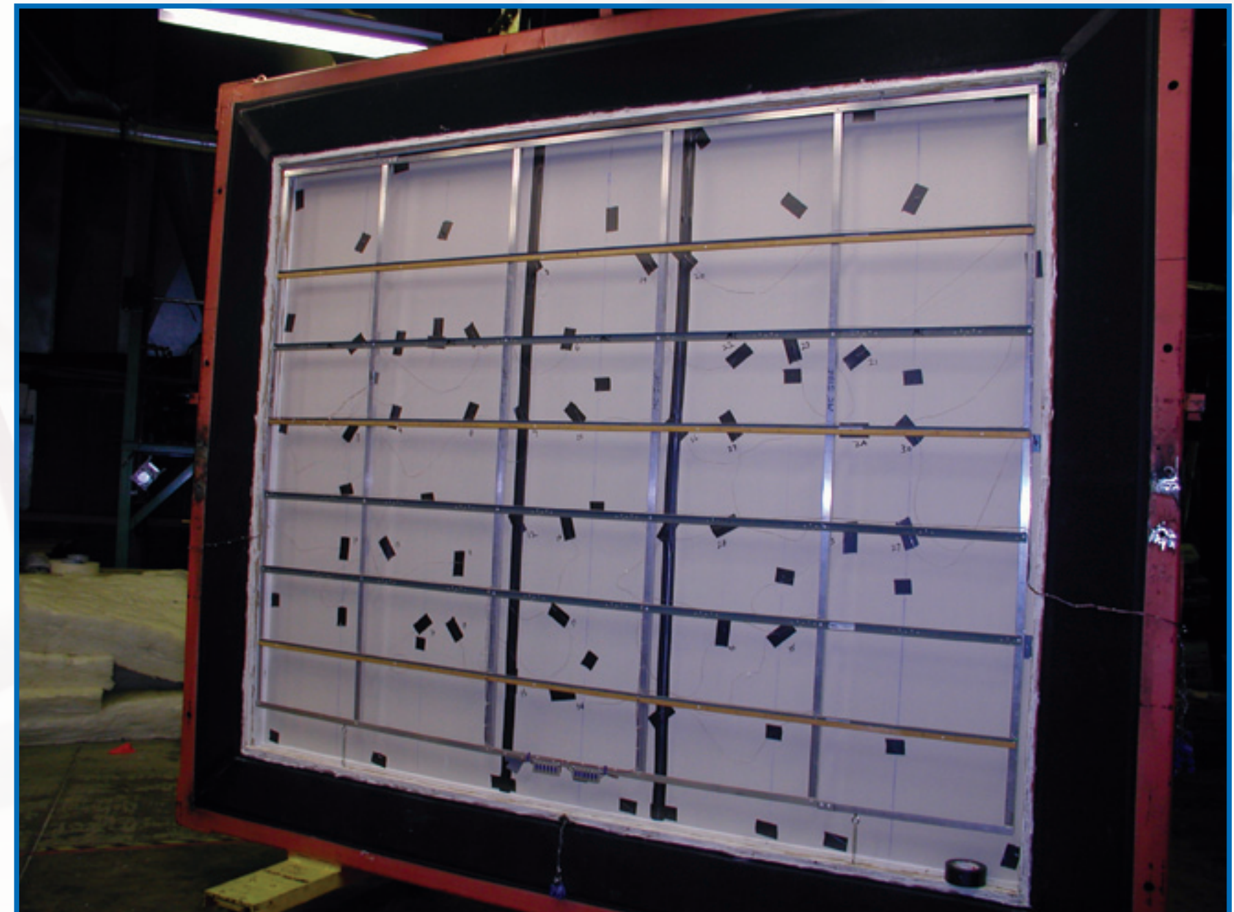
ASTM C1363: Interior side with gypsum wallboard and thermocouple grid
