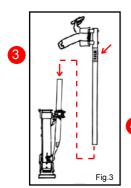
Read the yellow label on the upper strut tube. Keeping the strap buckles toward the toe of the stilt legs, slide the upper strut tubes down over the lower strut tubes and through the tube clamps. Position so the leg straps are just above the large portion of the leg calves. Note: Do not bend or "size" the leg bands. (Fig. 3-4)
