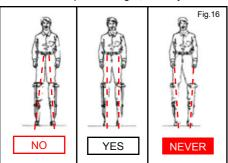
Loosen the bolts and nuts in the slotted brackets retaining the tube clamps. Slide the strut tube assemblies and clamps in the direction necessary to apply slight inward pressure to your legs. Securely tighten.
