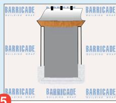
Install the bottom flashing over the wrap. Note: Barricade Building Products recommends the use of flashing material, such as OptiFlash® or Contour® premium butyl rubber flashing, that meets or exceeds Federal Specification UU-B-790a, Grade A and is minimum 6" in width.
