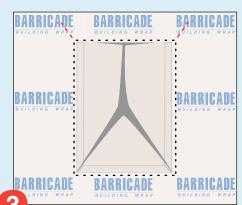
Make an inverted Y cut in the wrap at window rough opening. Make diagonal cuts at the top of the rough opening corners.
