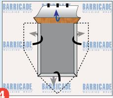
Fold the three flaps in through the opening, fastening them inside with staples set about every 6". Fold top flap up and tape temporarily as shown.
