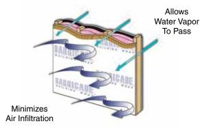
Barricade minimizes air infiltration while allowing moisture vapor to pass through it.
