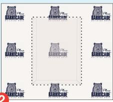
Secure Barricade Plus™ firmly in place by fastening it every 12"–18" along the vertical studs using large-headed or plastic cap nails or minimum 1" crown staples. You may install it over wood based, foam insulative, or fiberboard sheathing, and exterior gypsum board.
