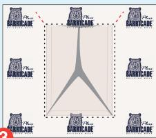
Make an inverted "Y" cut in the wrap at window rough opening. Make diagonal cuts at the top of the rough opening corners.
